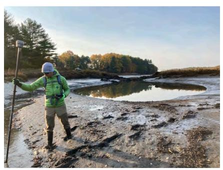
FIGURE 4.1 - Real-time kinematic GPS receivers are one of several tools that are typical of elevation surveys. Photo by Slade Moore.
