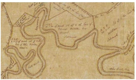
FIGURE 3.5 - Detail of a map documenting conditions before extensive channel modifications at Cascade Brook, Scarborough. The map was used extensively by diking companies to establish their rights to control water on the marsh.
