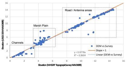
FIGURE 4.3 - Plot of surveyed ground elevations compared to topographic bathymetric elevation data classified by major cover class. Data from Namskatet Creek, Orleans, MA. Source: Woods Hole Group.
