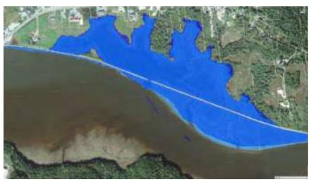
FIGURE 3.4 - Example of simulated present sea-level HAST inundation extent for existing site configuration (lighter blue) and proposed conditions (darker blue, barely visible at north margin).
