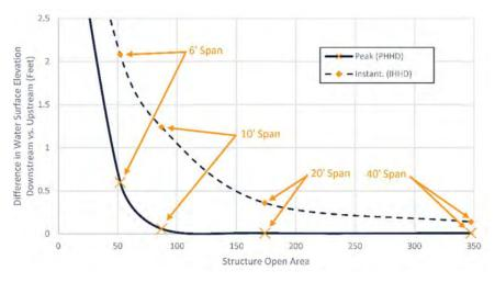
FIGURE 5.4 - Plot comparing HHD values calculated using PHHD and IHHD definitions, courtesy of Acadia Civil Works
