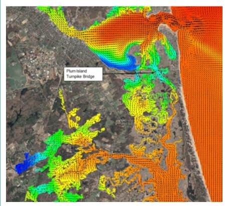
Flood simulation results showing color contours of salinity overlaid with current velocity vectors for a proposed widened Plum Island turnpike bridge opening in Great Marsh, Massachusetts. Blue tones represent low salinity, and red tones represent higher salinity.
